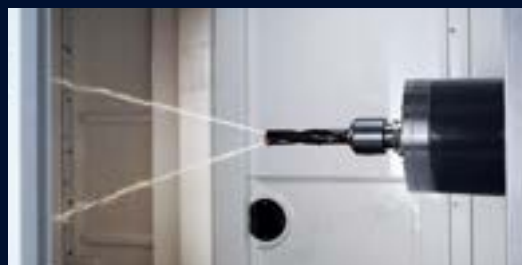
SPINDLE-THROUGH COOLANT (TSC) option
