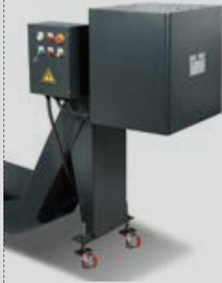
Scraper type drum chip conveyor
