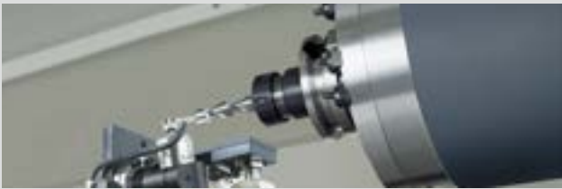
Automatic tool measuring device (TS 27R) option
