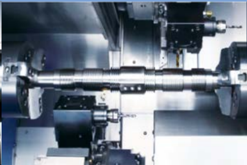
Different cutting processes can be carried out on a single workpiece using the upper and lower turrets simultaneously.
